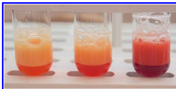
Figure 10. Three Alizarin Yellow tests on an oil with 2% free oleic acid. From left to right, the reagent (base plus indicator) was chosen to test for 0.8%, 1.6%, and 3.0% oleic acid. This low quality oil fails the first two tests, and only passes the third, as would be expected.
